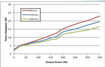
Figure 2: Power dissipation at nominal output voltage vs. load power for 90Vrms, 115Vrms and 140Vrms (60Hz) input voltage at Tb = 25°C.
