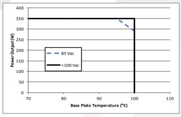
Figure 9: Output power vs. baseplate temperature derating curve
