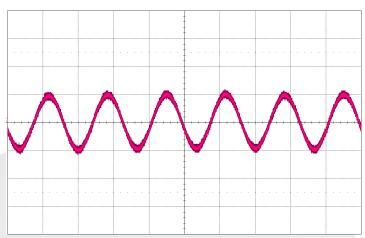
*Figure 7*: Output voltage ripple with 400μF Hold-up capacitor at full rated power (115VAC, 60Hz) Vout (5V/div), Timebase: (5ms/div)
