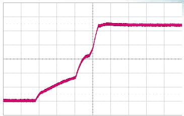
Figure 8: Output voltage startup waveform with 400uF hold-up capacitor, no load (115VAC, 60Hz), (50V/div), Timebase: (500ms/div)
