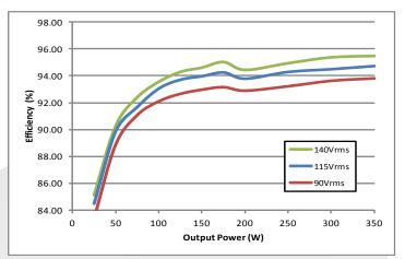
Figure 1: Efficiency at nominal output voltage vs. load power for 90Vrms, 115Vrms and 140Vrms (60Hz) input voltage at Tb = 25 °C.
